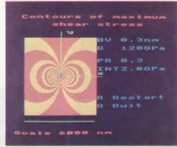
Fig 2. Map of the contours of maximum shear stress as a result of the elastic strain field around a single edge dislocation for a selected set of variables.
