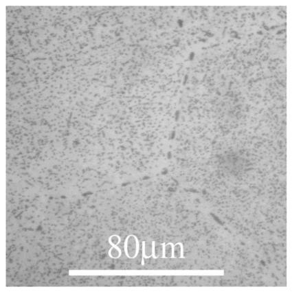
The  $\theta$  precipitates preferentially form on Al grain boundaries, as these are excellent heterogeneous nucleation sites.
