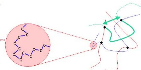
In this diagram, on the left each blue line represents a C-C link. The arrow shows the endto-end distance of the chain segment, depicted as a thickened line. The segments tend to coil up to some extent, rather than aligning in a straight line. This can be thought of as the system increasing its entropy. The probability distribution for the end-to-end distance can be
