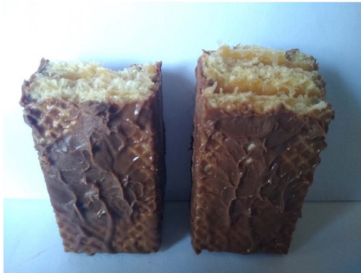
Figure 5. The fracture surface of the warm sample broken in a perpendicular orientation. Much of the surface actually tore and no flat surfaces could be seen. This results show a clear ductile fracture.
