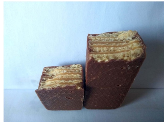
Figure 7. The fracture surface of the cold sample broken in a perpendicular orientation. The fracture surface is smooth and shiny, with the caramel and wafer fracturing. This results in a clear brittle fracture.
